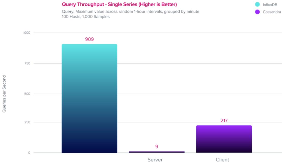
To reduce experimental variability, the query times were averaged over 1000 runs. With 1 worker threads we found that the worst-case mean query response time with server aggregation for **Cassandra was 106ms (9 queries/sec)**. The same query took an average of **1.1ms (909 queries/sec) for InfluxDB**, and **4.6ms (217 queries/sec)** when doing client-side, application-level data aggregation for Cassandra, which required custom development as mentioned above.
