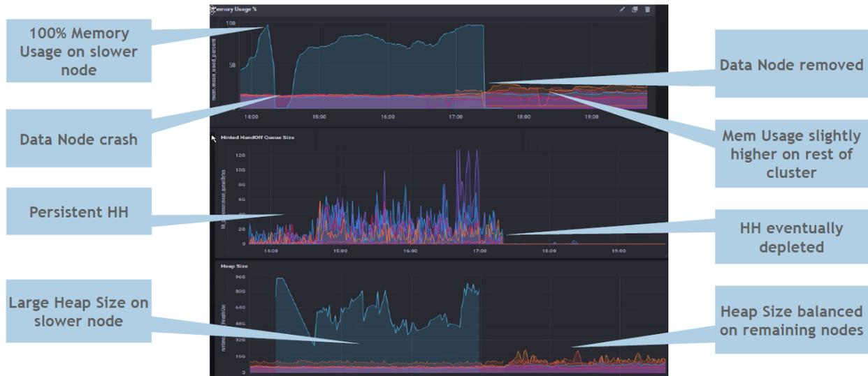
While the slower node is in the cluster, the hinted handoff was persistent. All of the nodes in the cluster were trying to send to that one slower node. Hinted handoff queue buildup occurred on the rest of the nodes in the cluster. Also, the slower node had a larger heap size, trying but unable to keep up with all the writes coming to it.
