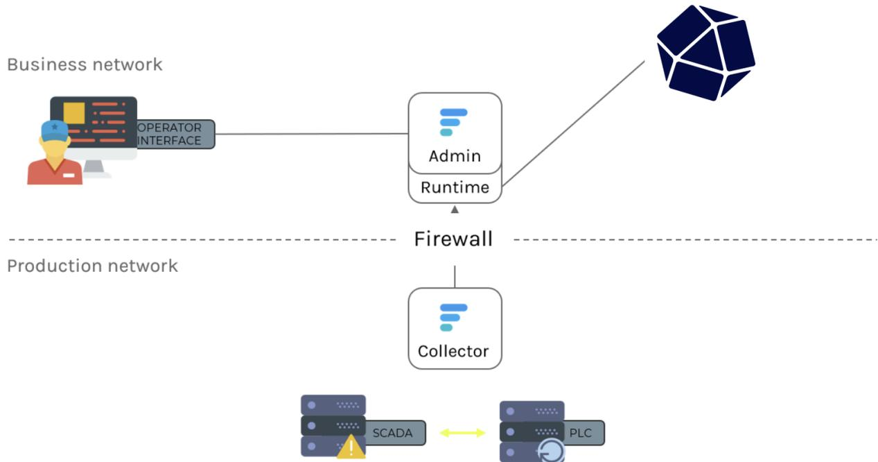
Factory’s collectors collect data from PLC data systems that are controlling the process and forward it through the firewall towards an API component that sits in the business network.
