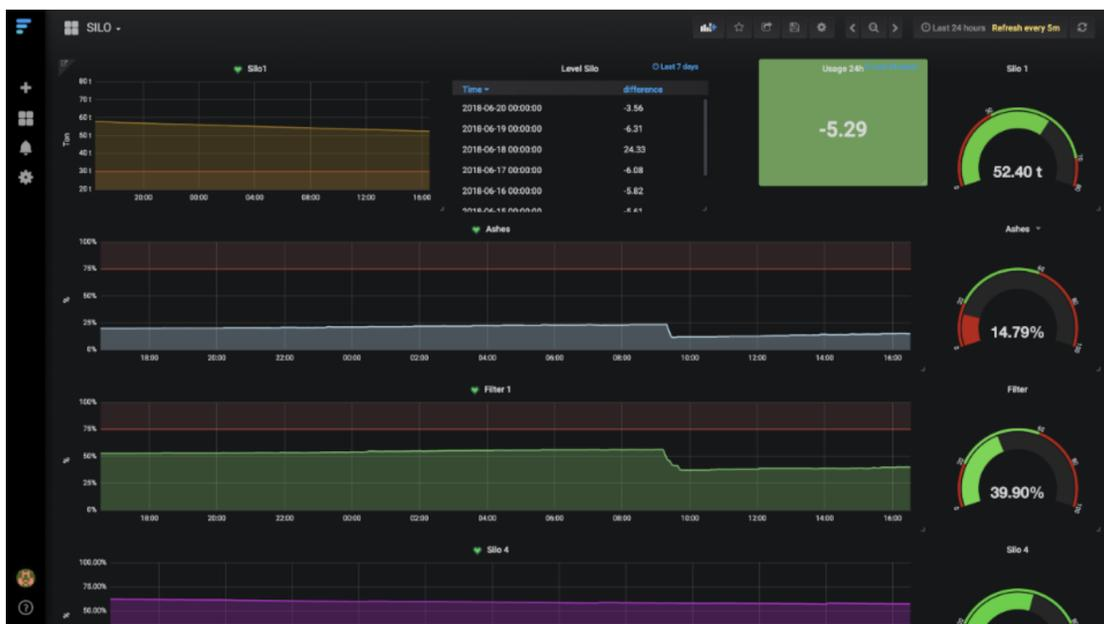
Adding to that, an early benefit that A&S gained with the new ‘transparency’ of process data was the ability to detect early signs of tank leakage, which prevented costly unplanned downtime.
