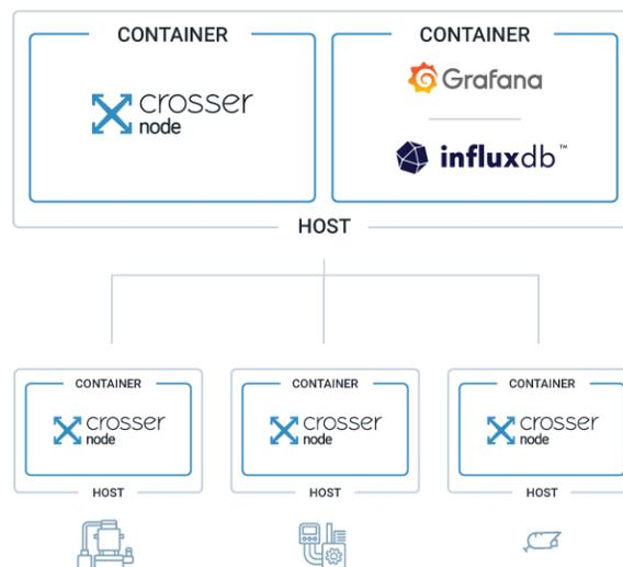
This scenario deploys a Crosser node on (or near) each data source so each node only collects and processes data from a single source. These distributed nodes then transmit data to a centralized deployment of InfluxDB for storage and Grafana for visualization. Deploying another
