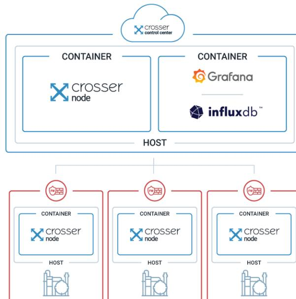
This configuration is similar to the scale-out iteration, but instead of hosting InfluxDB, Grafana, and the optional Crosser node on-site, they live in the cloud. The distributed Crosser nodes collect and analyze data locally but transmit data to the cloud where users can aggregate data across multiple facilities for a global view of operations.
