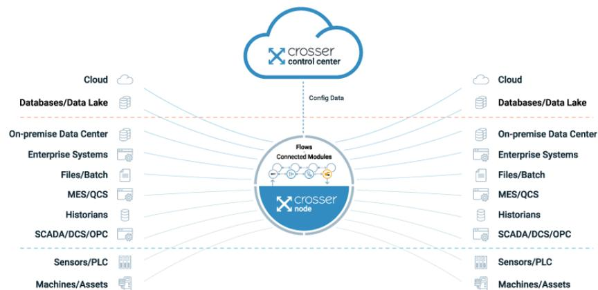
Crosser Control Center is the platform's orchestration and management layer. One of the key tools in Crosser Control Center is the Flow Studio, which is a visual interface that enables users to design custom data workflows using pre-built modules. These modules include common IIoT protocols, like [MQTT](#), [OPC UA](#), [Modbus](#), and more. Users can parameterize these flows so they can work dynamically with different input sources but create consistent output.
