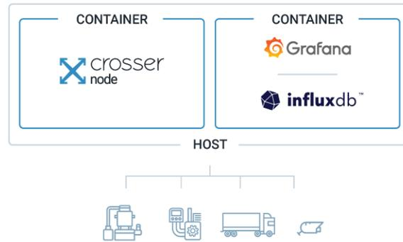
This scenario deploys the data historian containers on a single local host. It provides a local UI and uses a single Crosser node for pre-processing and historical analysis. This is something that users might want to install on a per unit, area, or facility level.
