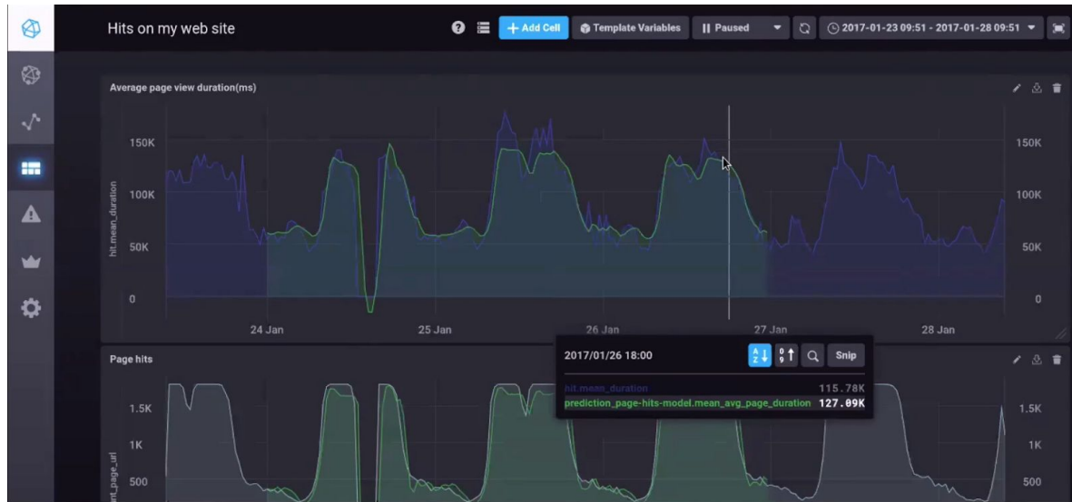
Visualizing Loud ML predictions in Chronograf using InfluxDB as the data source
