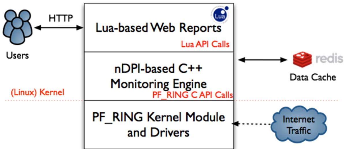
The ntopng Monitoring Engine is coded in C++ and based on the concept of flow (set of packets with the same 6-tuple). Flows are inspected with a home-grown DPI library named nDPI aiming to discover the “real” application protocol (no ports are used). Information is clustered per (Capture) Network Device, Flow, and Host.
